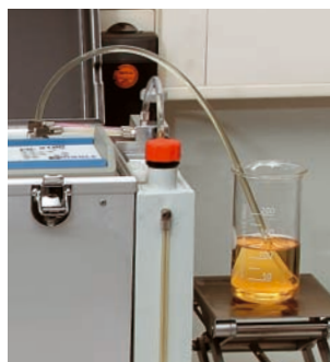
Particle counter type Pic 9100 which is used by Zeller+Gmelin.
